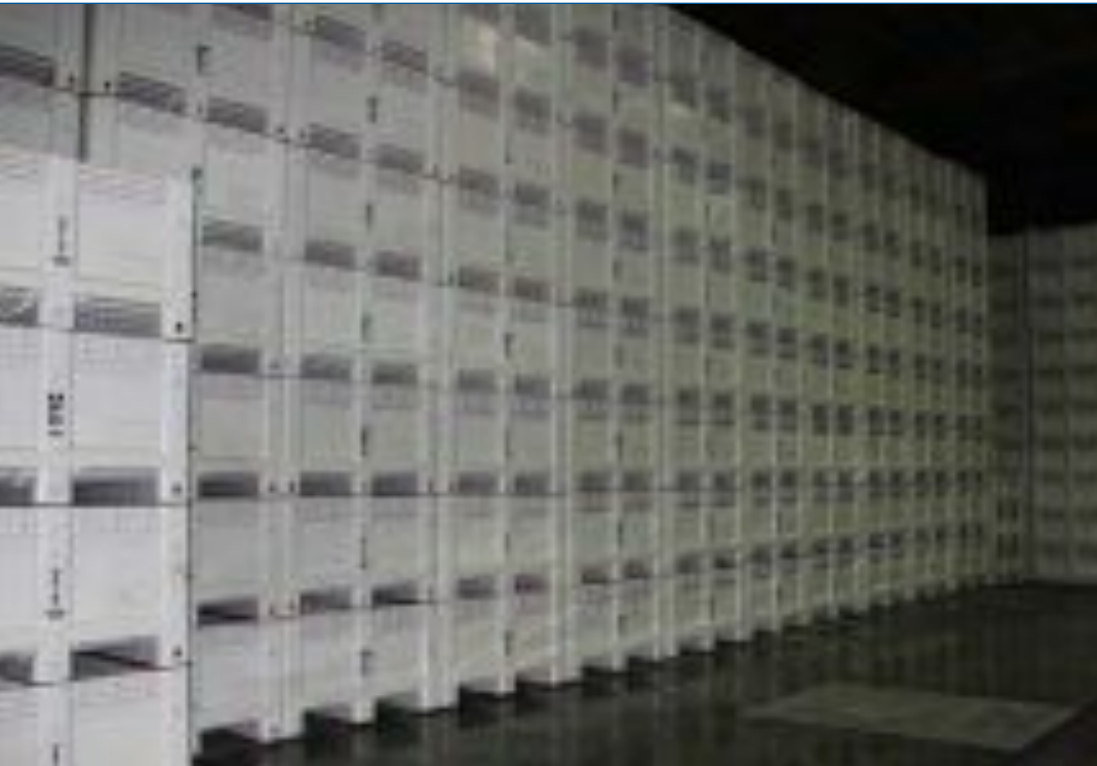
STORAGE CAPACITY DOUBLED WITH AN INCREASED STACK HEIGHT OF 8 PROBIN 24-S PER COLUMN
